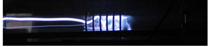
Fig. 6. Intermediate formation stage of the argon plasma.
