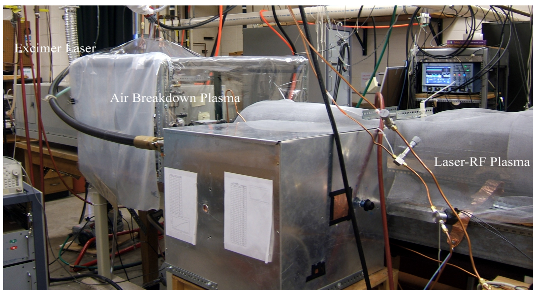
Fig. 2: Photograph of the high-pressure plasma arrangement. Both the laser focused air breakdown system and the high pressure laser-RF plasma system are aligned with the excimer laser so the two experiments can be carried out in tandem.
