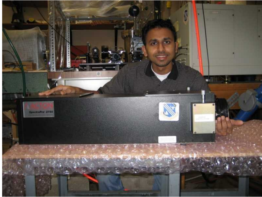
Fig. 16: The spectroscopy system: monochromator (Acton Research, Model: ARC-SP-2758) and ICCD (Andor iStar, see Fig. 12).
