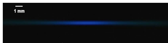
FIG. 5. (Color online) 193 nm laser induced plasma image captured with 75 mm focal length lens.
